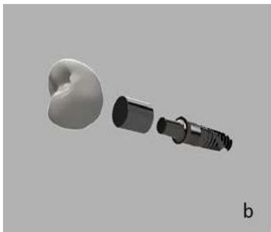
Fig. 1 – Experimental models: a) Model with polyetheretherketone (PEEK) characteristics; b) Model with cobalt-chromium alloy characteristics.
