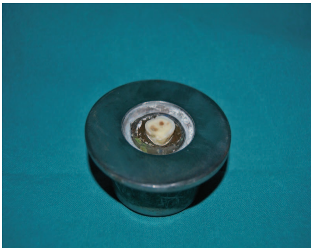
Fig.1 Custom made grinding cylinder.
