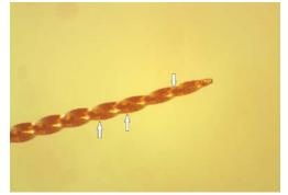
Fig. 5 – Apical third of Kerr file instrument after mechanical cleaning method (red spots, white arrows).
