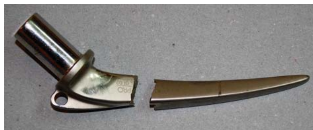
Fig. 9 – Endoprosthesis body fractures due to material fatigue.
