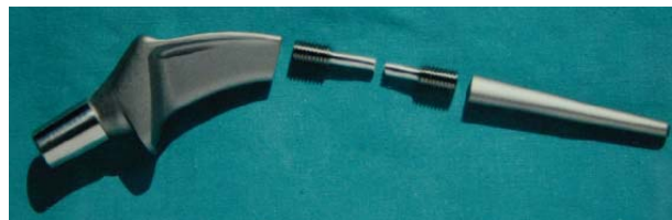
Fig. 7 – A test specimen resulting from cutting the physical model out.
