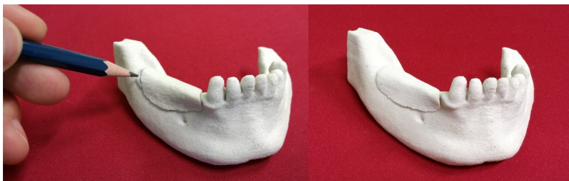
Fig. 7 – Physical models of the lower jaw generated by the rapid prototyping RP technology.
